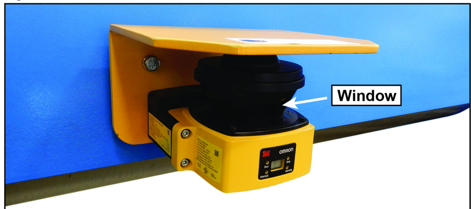
Figure 7: Laser Scanner Window Location
